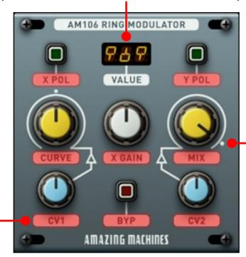
The white dots that circle around the CURVE and MIX knobs are Modulation Indicators, they move away from the knobs indicators depending on how the CV1 and CV2 Inputs are set.
